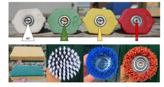
Cleaning utensils in the »ROBUST«-project: The top shows the attachments for the highpressure water jet, which are characterized by a different jet angle.
