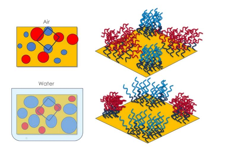
Schematic illustration of a surface consisting of hydrophilic and hydrophobic domains of a fouling-release mechanism. Momentive Performance Materials GmbH
