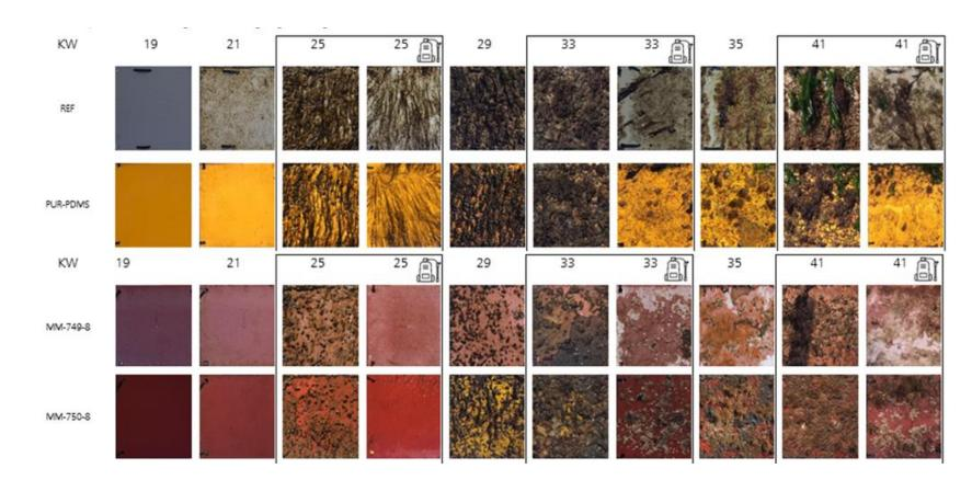
Fouling scenario for three selected Helgoland wear samples in 2022 as a function of time, masked by calendar weeks. The framed boxes show the sample before and after cleaning with high pressure water jet. The upper row of photos depicts the commercial reference, which accumulates significantly more fouling and has a lower cleaning success. © Fraunhofer IFAM
