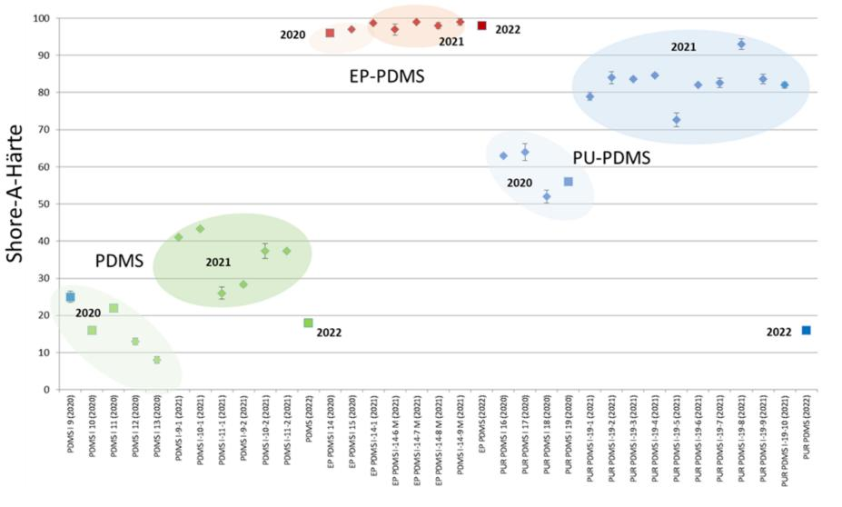
Comparison of Shore-A-hardness for PDMS, EP-PDMS and PU-
