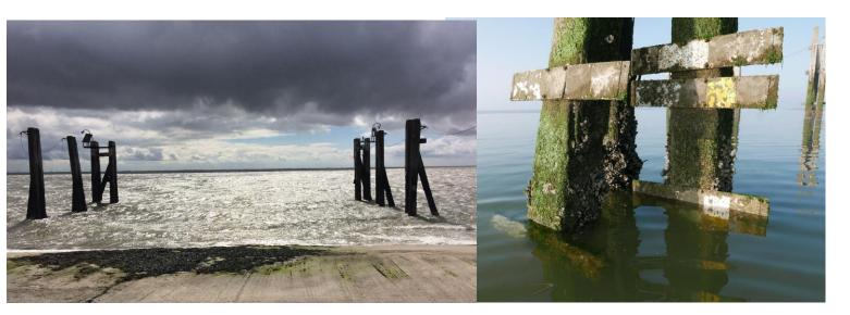
Brill station at the North Sea island of Norderney, Germany (53°41'47.8"N 7°09'25.5"E) Samples are immersed here in the intertidal zone as well as permanently submerged
