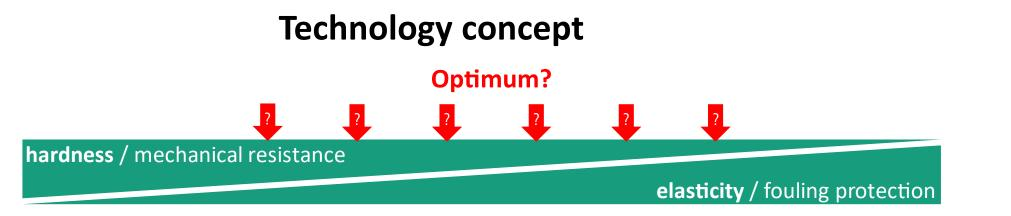
Conversion of the silicone system with low mechanical resistance while retaining the foul-release properties into an abrasionresistant cleanable coating
