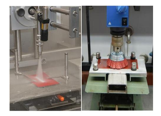
High-pressure water jet (left) and the in-house development of a brush laboratory test rig (right) for pre-qualification of the developed systems. The pre-selection was necessary in order to make the most effective use of the limited number of test sites in the field.  $\bigcirc$ Momentive Performance Materials GmbH
